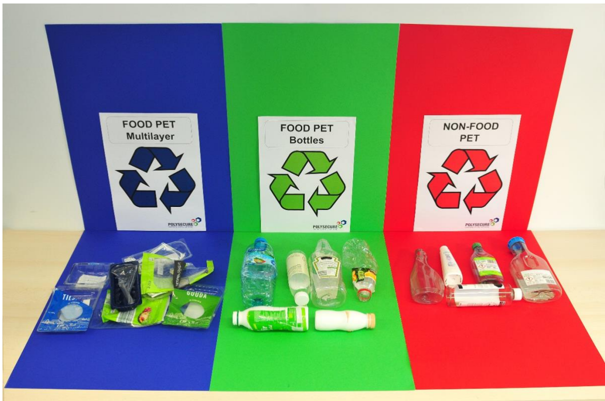
Example of different PET-based packaging fractions that could be differentiated and thus sorted by tracers (Photo credit: Pforzheim University)
